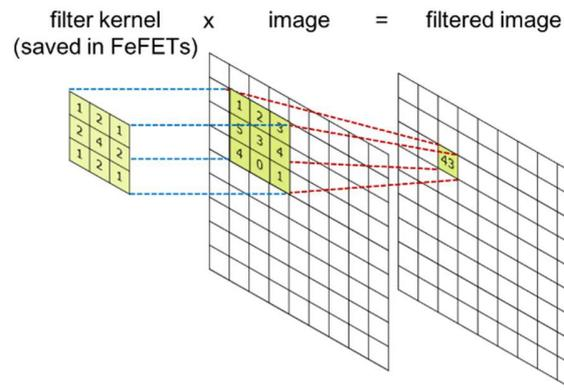
**Figure 3** Schematic of image application showing the filter kernel convolution with the input image to produce a real-time filtered result.
