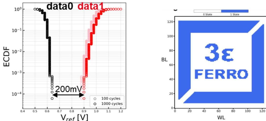
**Figure 1** Initial characterization of 16k FeRAM array on MD200v3 lot showing (left) the memory window to 4s and (right) the zero bitfail after 1000 cycles performed on the word vs. bitline  $128 \times 128$  memory array storing the 3εFERRO logo (to be published).
