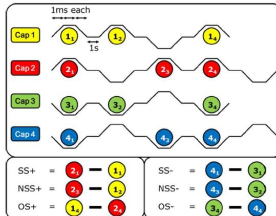
**Figure 2** Methodology first developed by Texas instruments for endurance/retention tests of ferroelectric capacitors, considering the polarization state and switching history [Rodriguez Trans Device Mater. Reliability 4, (2004)].
